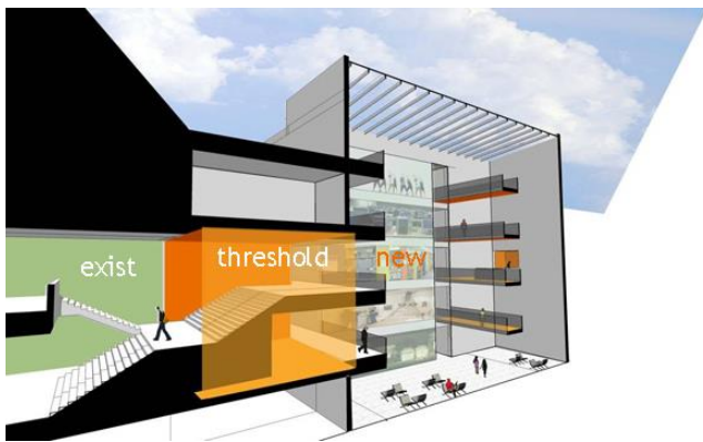
Figure 4. WJB section illustrating the original dining hall (on the left), threshold area, and the new addition (on the right) defined by the 5-story open atrium. Drawing courtesy of Gould Evans Architects.
